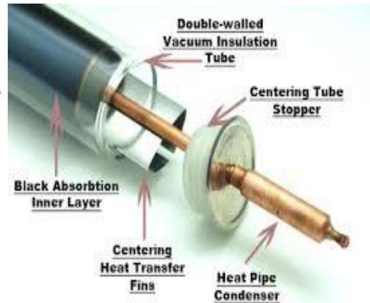
Fig. 1-b- Evacuated Tube Heat Pipe
